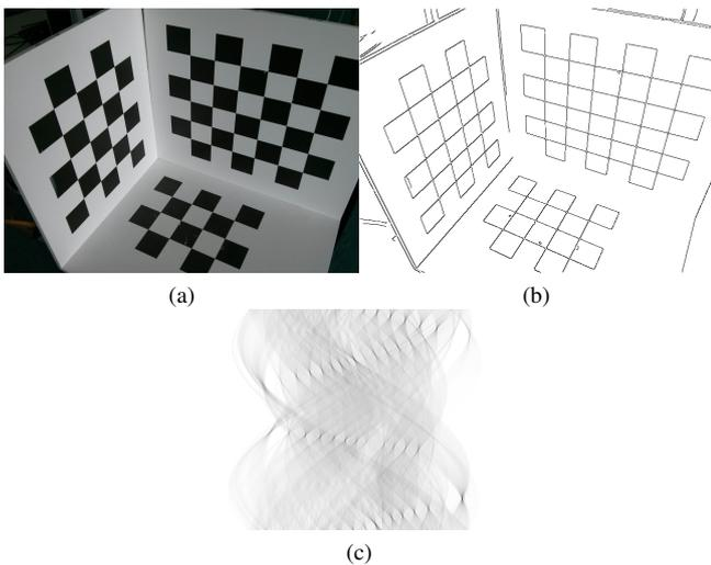
Fig. 15: Exemplary output images of the demonstrator system; (a) input image (640x480 pixels); (b) edge image (640x480 pixels); (c) parameter space (512x320 pixels)
