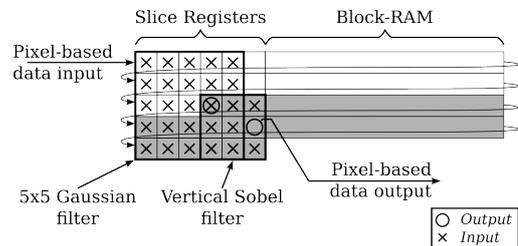
Fig. 4: Exemplary *2D Window Pipeline*, implementing Gaussian filtering and the Sobel operator
