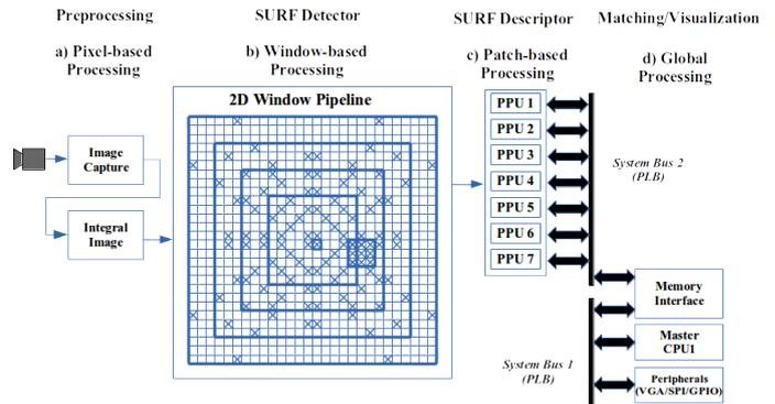
Fig. 13: Structure of the object recognition system, fully integrated in a single Spartan-6 LX150 FPGA
