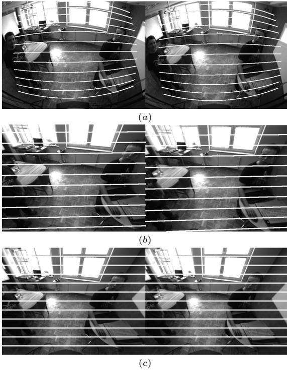
Fig. 5: Example images showing raw (a), undistorted (b) and rectified (c) image pairs of a stereo camera setup
