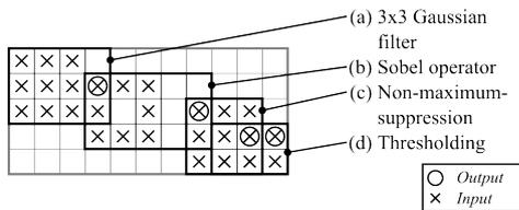
Fig. 9: Structure of the Canny edge detection module
