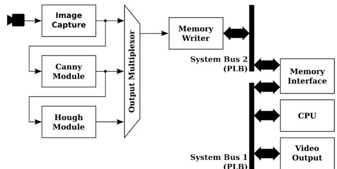
Fig. 14: Structure of the demonstrator system for the *Canny Module* and the *Hough Module*
