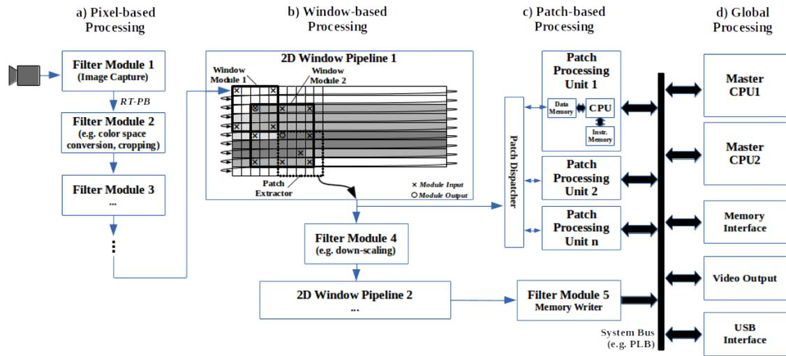
Fig. 2: Exemplary structure of an image processing system
