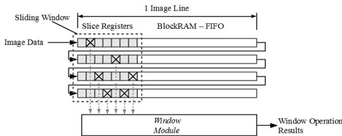
Fig. 3: Principle of the sliding window technique
