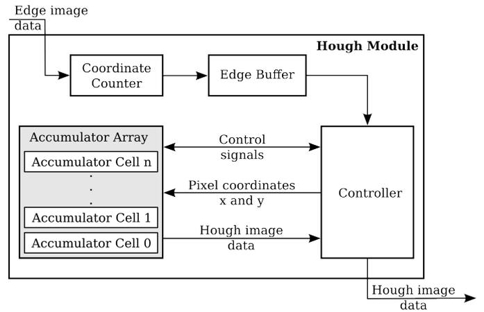
Fig. 10: Structure of the *Hough Module*
