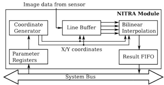
Fig. 7: Structure of the *NITRA* module for real-time non-linear image transformations
