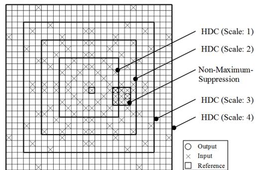
Fig. 8: Structure of the *SURF* detector module, used for real-time natural feature detection
